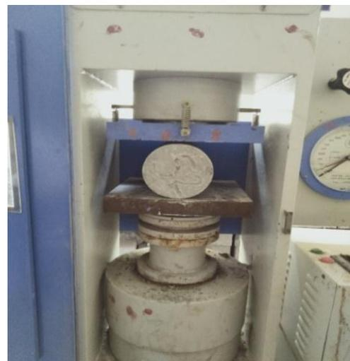
Figure 2. Split Tensile Strength Machine
