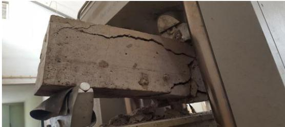
Figure 6. Failure Mode of Beam-3
