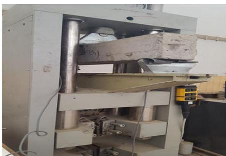
Figure 4. Beam set up on universal Testing Machine
