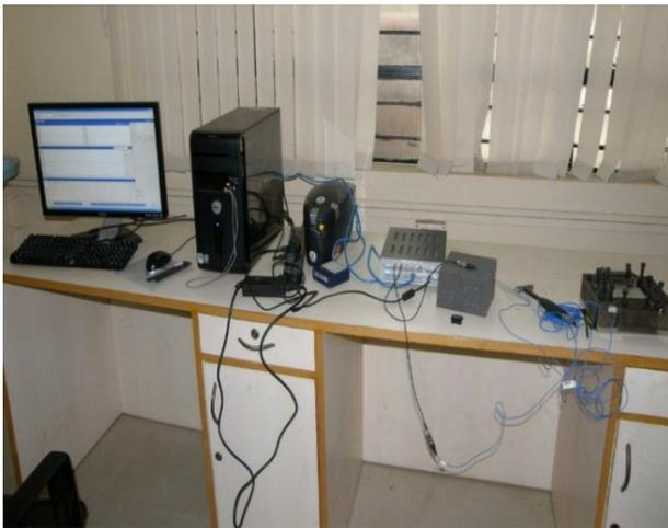
Fig. 3. experimental setup for vibration testing of the sandwich specimens with Data acquisition System
