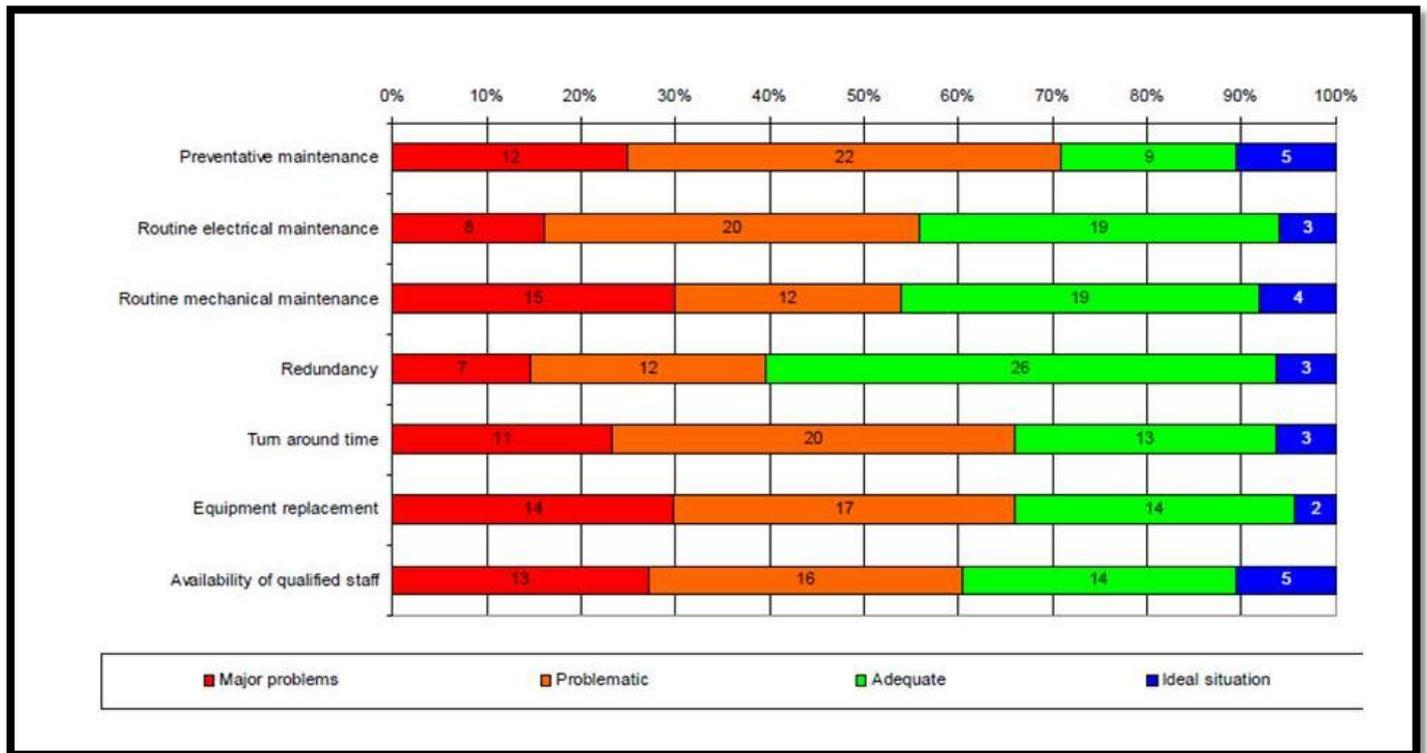
**Figure 4:** Statistics on the operational state of various wastewater treatment plants (Snyman et al.,2006)
