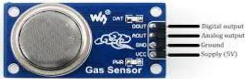
**Fig:** Gas sensor (MQ-135)
