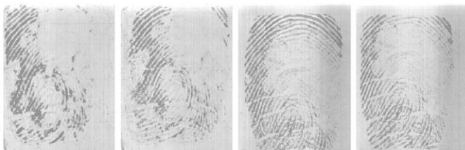
Fig 8. An example of “failure to enroll” for fingerprints (with respect to a given fingerprint recognition system): four different impressions of a subject’s finger exhibiting poor quality ridges due to extreme finger dryness. A given fingerprint system (using a certain sensor and matching algorithm) might not be able to enroll this subject since minutiae and ridge information cannot be reliably extracted.
