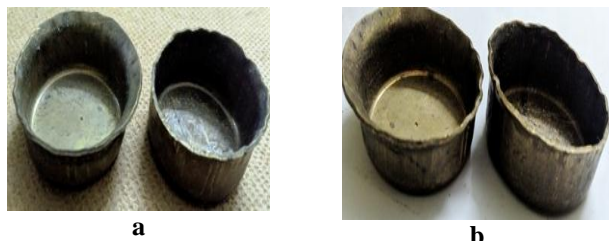
Fig. 5 Deep drawn cups of brass sheets a) with heat treatment b) without heat treatment
