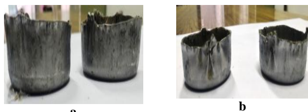
Fig. 4 Deep drawn cups of SS304 a) with heat treatment b) without heat treatment
