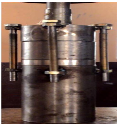
Fig.2 Experimental Setup of Angular deep drawing
