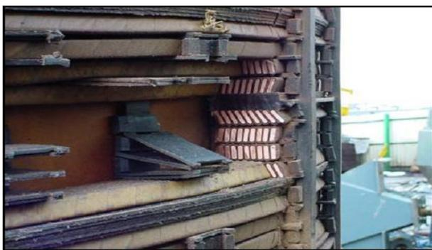
Fig.5 Tilting under an axial load [9]
