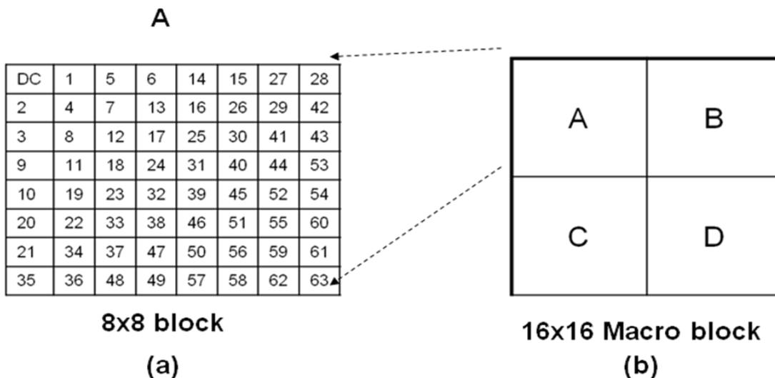
Figure 2. 16x16 Macro block into four 8x8 sub blocks
