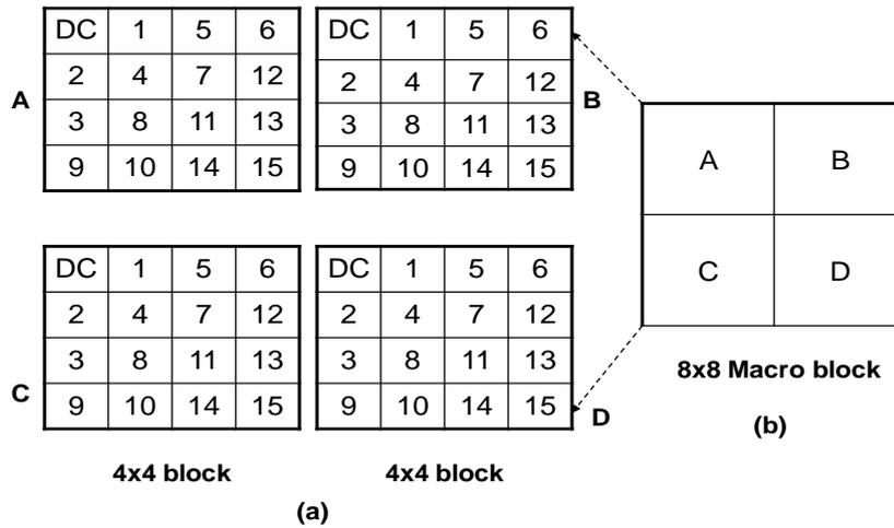
Figure 1. 8x8 Macro block into four 4x4 sub blocks
