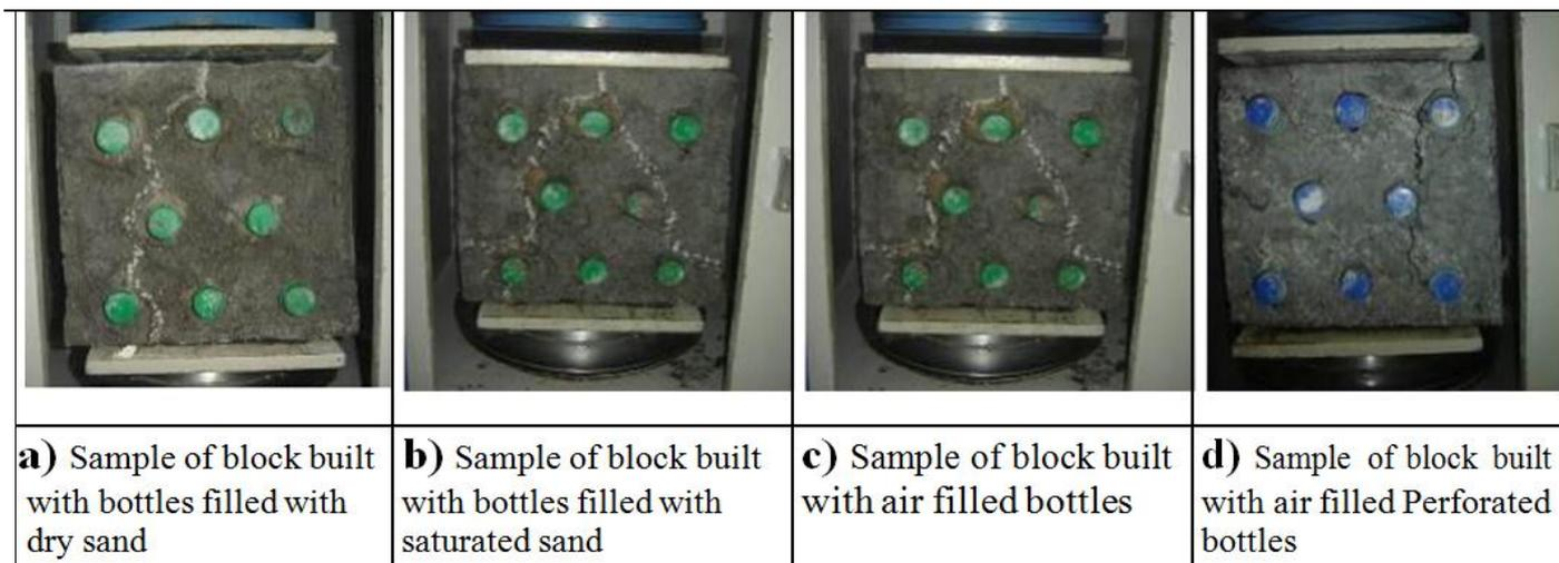
**Figure 2** Arrangement of bottles in the block (filled with different sands and air)
