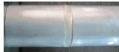
Figure 5 A welded pipe by the UFSWoP process.
