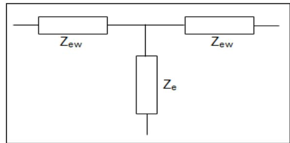
**Fig. 4:** Three-way current split based on impedance
