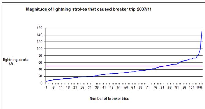
Fig 16: Incident of breaker interruptions vs stroke magnitude
