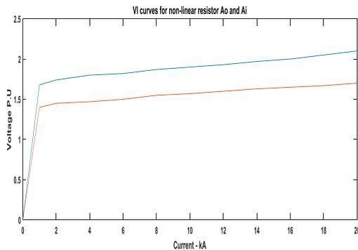
Fig 11: V-I non-linear characteristic for A<sub>0</sub> and A<sub>1</sub>
