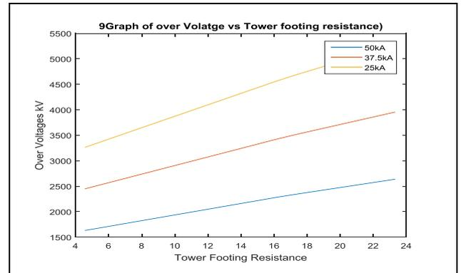
**Fig 9:** Enhance earthing (less than 30ohms) vs over voltages
