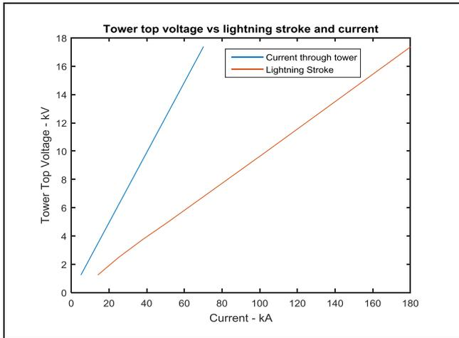
**Fig 6:** Tower Top voltage vs lightning stroke
