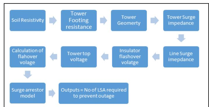
**Fig 1:** Process flow diagram to determine required number of surge arrestors to prevent power interruptions.
