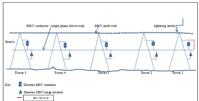
Fig 12: Surge arrester connected on a parallel on a number of towers
