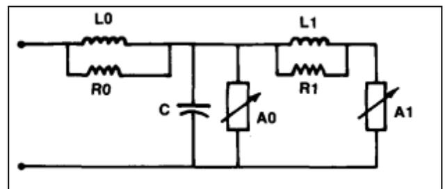
**Fig 10:** IEEE frequency-dependent model line arrester
