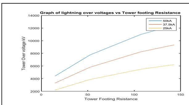
**Fig 8:** Tower Top Voltage variation vs Tower Footing Resistance
