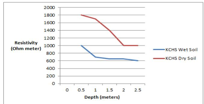
Fig 3: Soil Resistivity test at KCHS
