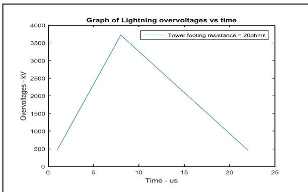
**Fig 7:** Over voltages caused by a 37.5kA lightning stroke
