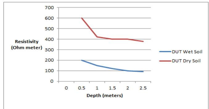
Fig 2: Soil Resistivity tests at DUT
