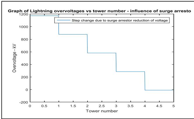
**Fig 13:** Lightning over voltages vs tower number – influence of surge line arrestors
