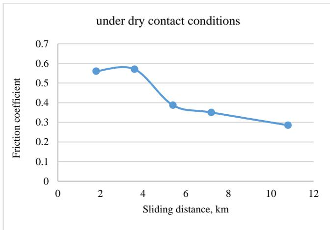
**Fig. 3.** Friction coefficient of UHMWPE under dry contact conditions
