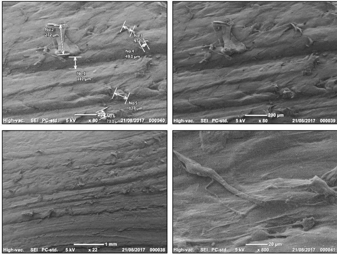
**Fig. 8** SEM observation on UHMWPE under dry conditions
