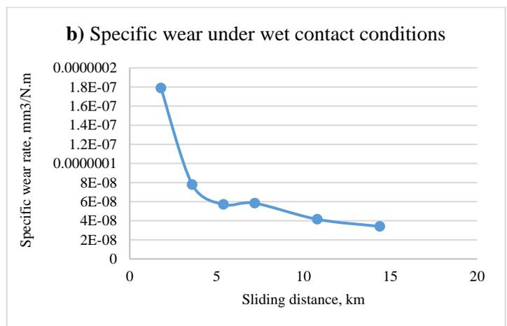
**Fig. 4.** Weight loss and specific wear rate of UHMWPE under wet contact conditions
