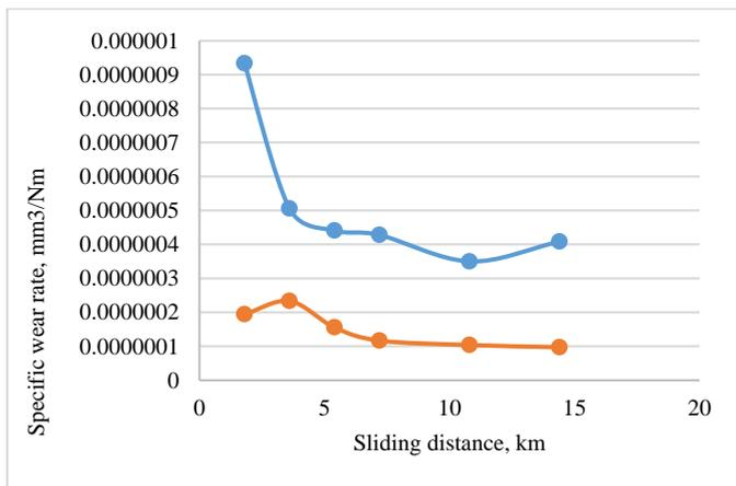
**Fig. 6.** Wear results of UHMWPE under dry and wet conditions
