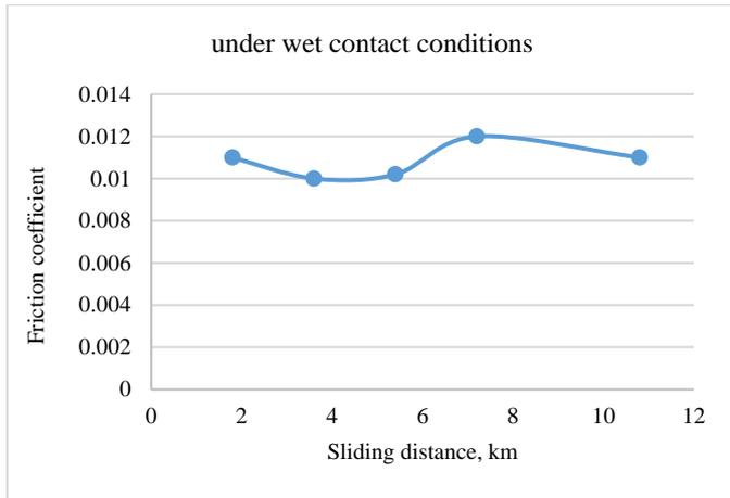
**Fig. 5** Friction coefficient of UHMWPE under wet contact conditions
