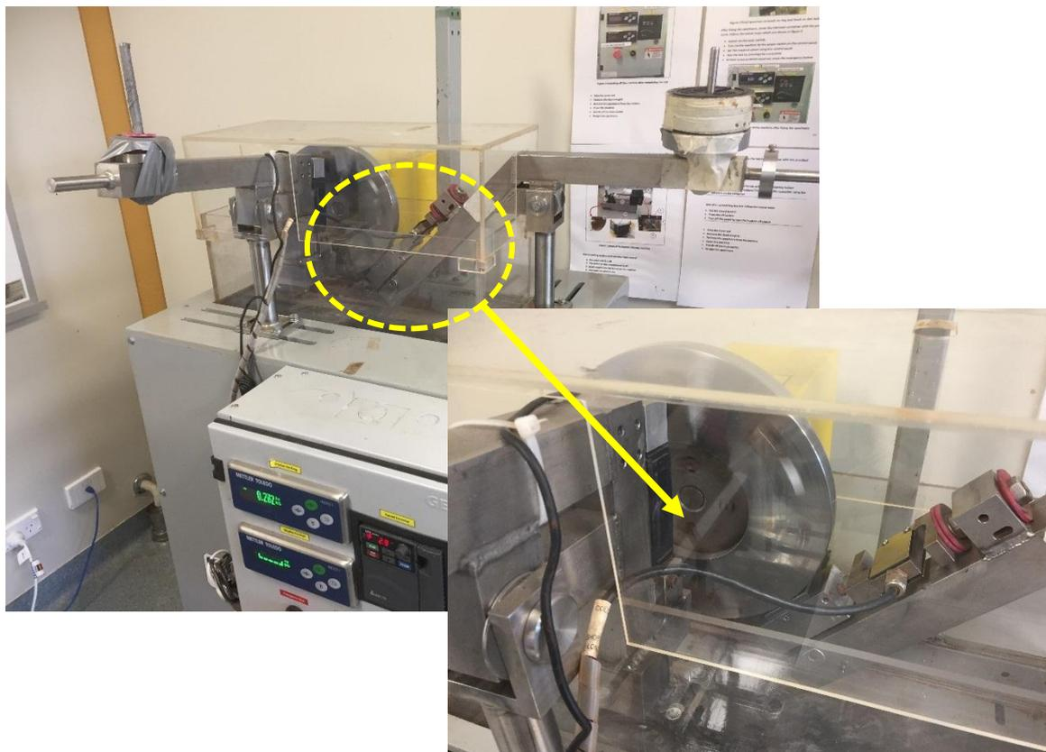
**Fig 1.** Tribology machine and zoom area of the interface of block on ring configuration
