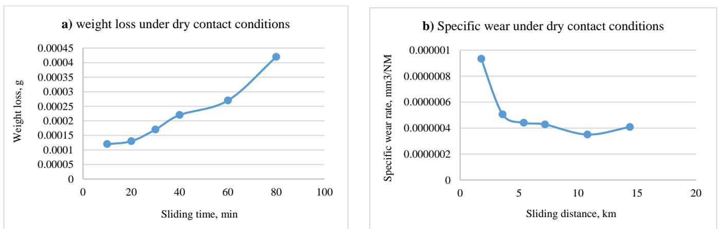
**Fig. 2.** Weight loss and specific wear rate of UHMWPE under dry contact conditions
