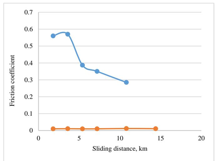
**Fig. 7** Frictional results of UHMWPE under dry and wet conditions
