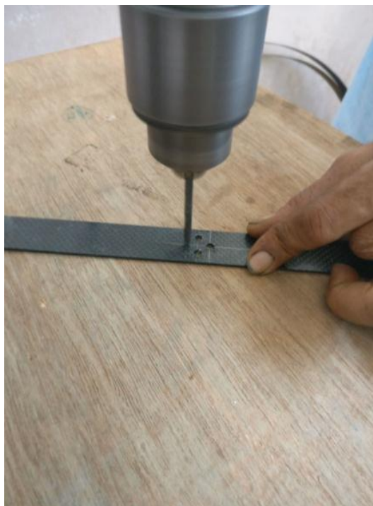
Figure 5. Drilling of holes
