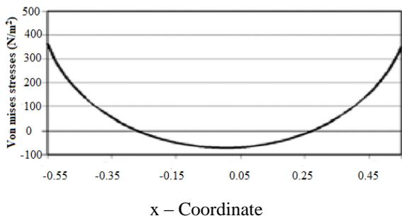
**Fig. (11) Von Mises stresses along x-coordinate at thruster Load in x – direction.**
