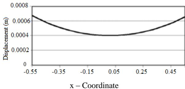
**Fig. (16) Displacement along x - coordinate at thruster Load in x – direction.**
