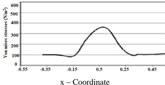
**Fig. (12) Von Mises stresses along x-coordinate at thruster Load in y – direction.**
