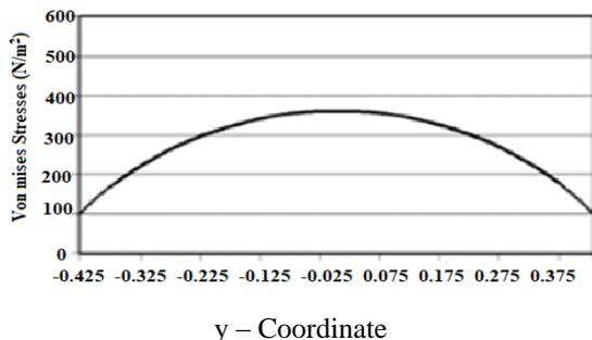
**Fig. (13) Von Mises Stresses along Y-coordinate at thruster Load in x – direction.**
