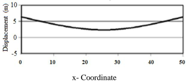
**Fig. (19) Displacement a long x – coordinate at thruster Load in y – direction.**
