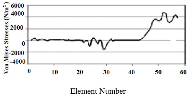
**Fig. (10) Von Mises Stresses Viruses Element Number at thruster Load in x – direction.**
