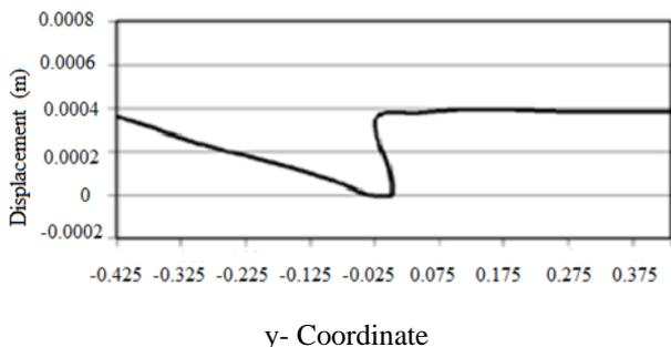
**Fig. (17) Displacement along Y-coordinate at thruster Load in y – direction.**
