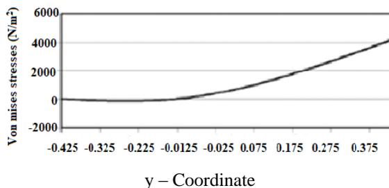
**Fig. (14) Von Mises Stresses along Y-coordinate at thruster Load in y – direction.**
