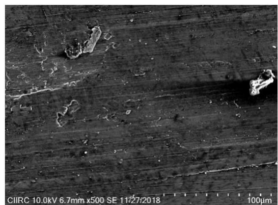
Fig-10: Worn out surface of 6061 aluminium alloy reinforced with 1.5% CNT under 300rpm
