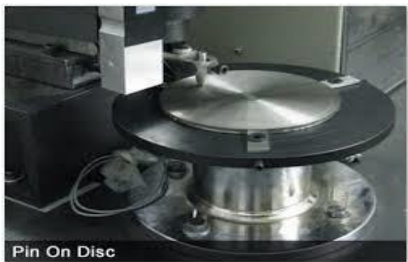
Figure 5: pin-on-disc test apparatus
