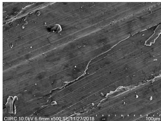
Fig-12: Worn out surface of 6061 aluminium alloy reinforced with 1.5% CNT under 700rpm
