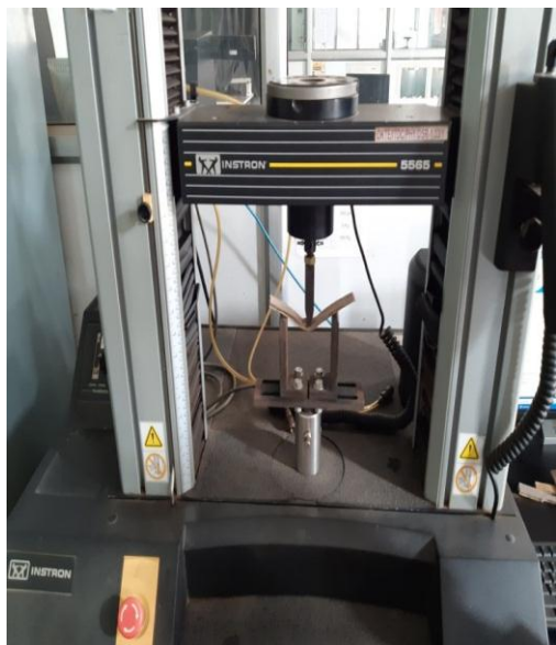
Fig.12 Bending test set up on INSTRON 5565 machine
