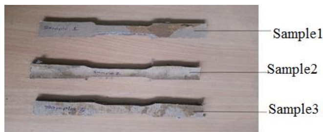
Fig.5 Tensile test specimen before testing (ASTM D638)
