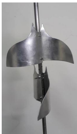
Fig. 28. Two stages 2CW with perpendicular orientation two blades IceWind turbine.
