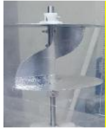
Fig. 24. Two end plates with two reversed blades IceWind turbine.
