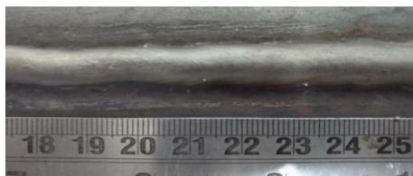
**Figure 1(a):** Hardfaced layer- Sample-1
