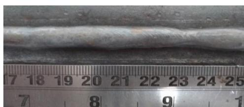
**Figure 1(c):** Hardfaced layer- Sample-3
