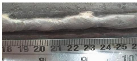
**Figure 1(b):** Hardfaced layer- Sample-2
