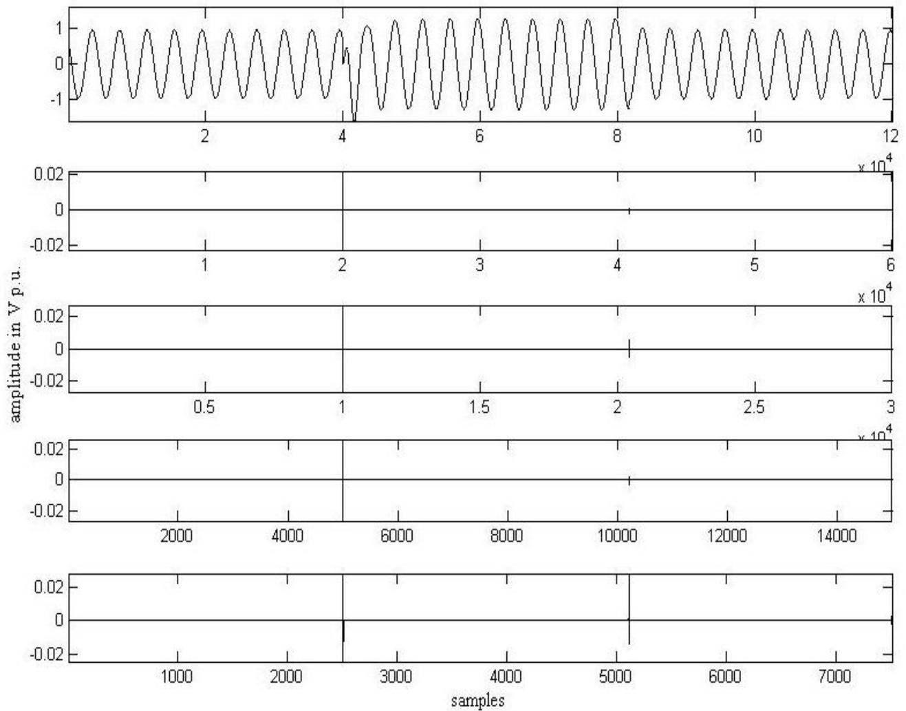
**Fig. 4:** Decomposition of pure sine wave with swell using DWT
