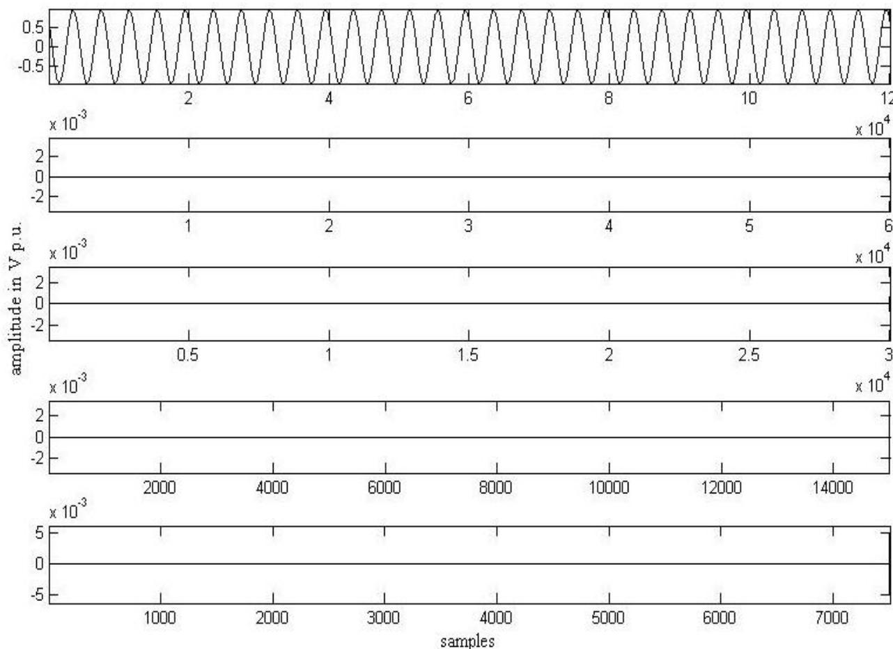
**Fig. 2:** Decomposition of pure sine wave using DWT
