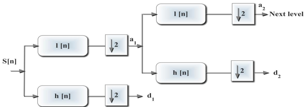
Fig.2. Block diagram of DWT decomposition
