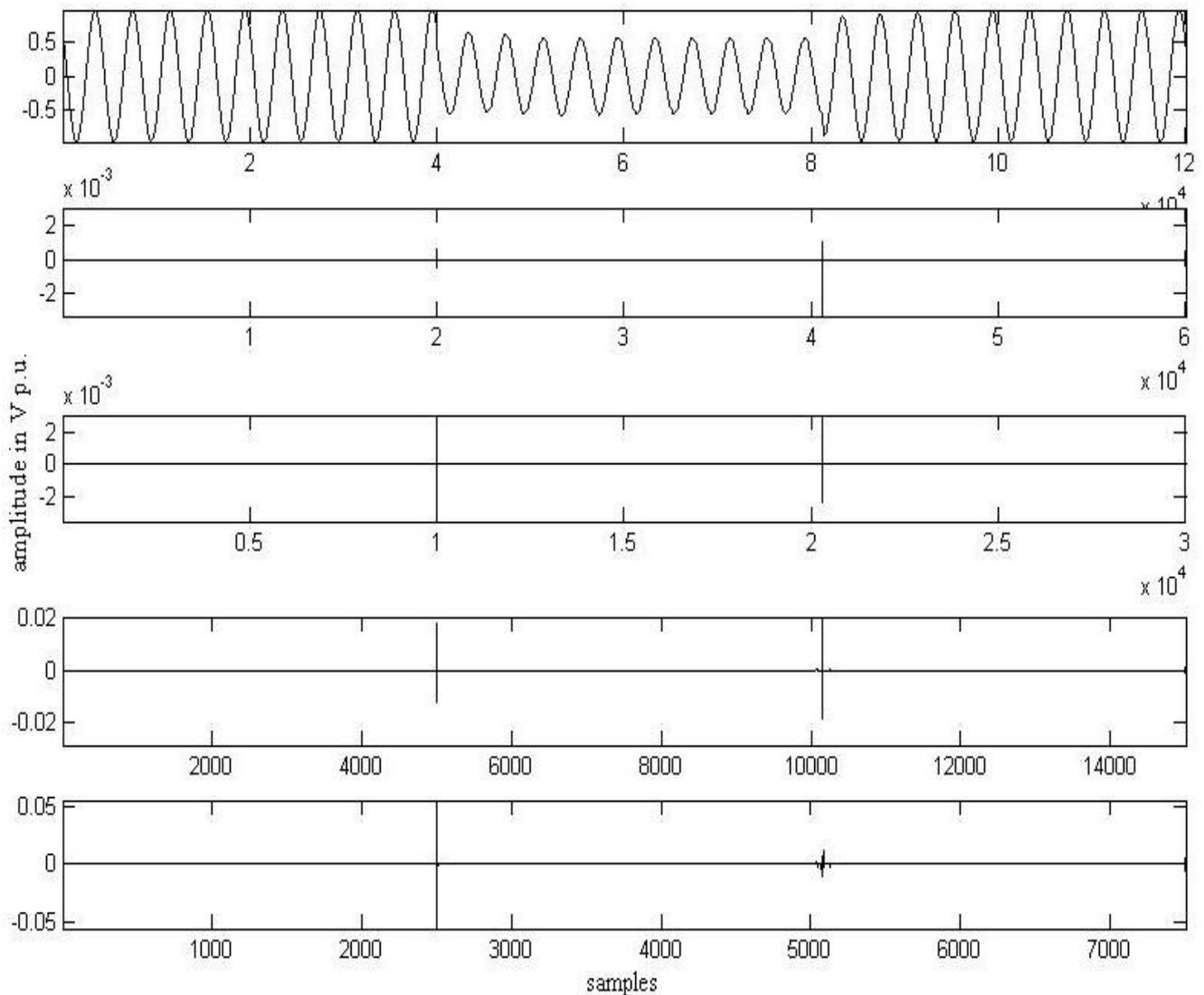
**Fig. 3:** Decomposition of pure sine wave with sag using DWT
