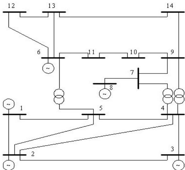
**Fig. 1:** Single line diagram of IEEE 14 Bus Test System
