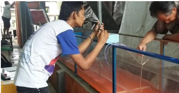
Fig 2. Water depth and velocity measurement for 12 section (source: primary data)
