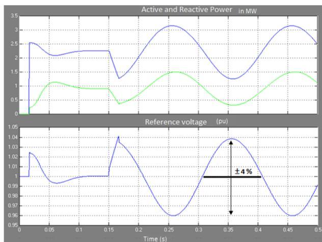
**Figure 2:** Active, reactive power and reference voltage with dynamic load
