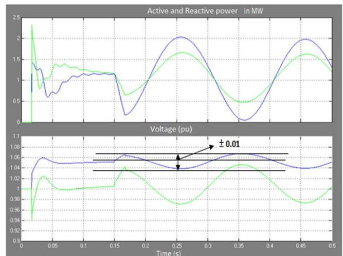
**Figure 3:** Active, reactive power and reference voltages with dynamic loads and REG integration
