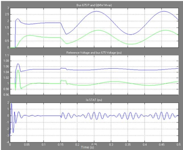
**Figure 4:** Active, reactive, reference voltage and STATCOM modulated current
