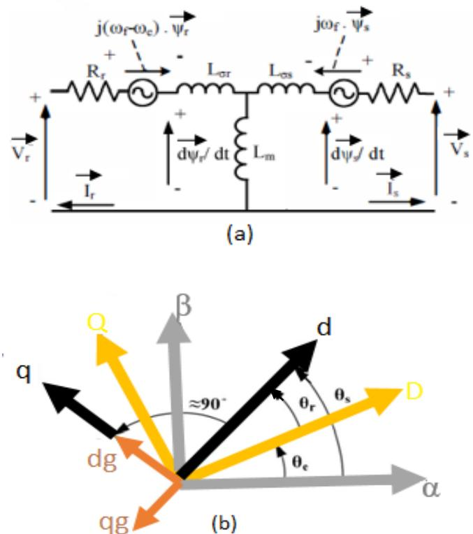
**Figure 1.0:** (a) Electrical model of (b) DFIG Relation among different reference frames
