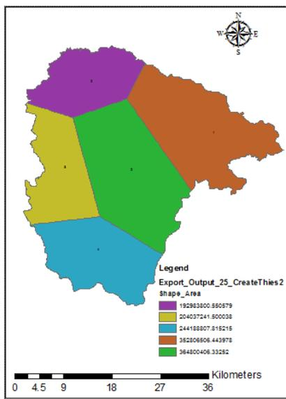
Fig 3 Thiessen polygon of study area for 5 rain gauge station
