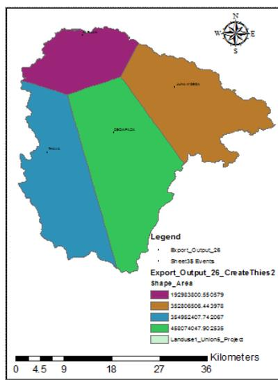
Fig 4 Thiessen polygon of study area for 4 rain gauge station
