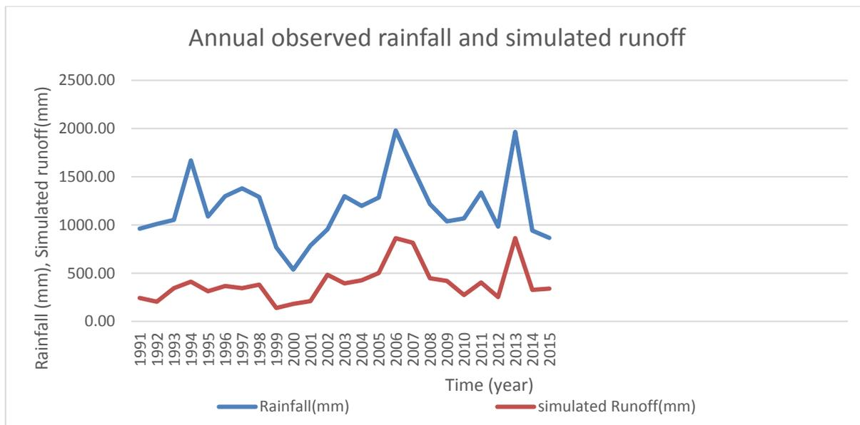
**Fig 7:** Annual Rainfall and Simulated runoff by SCS-CN method
