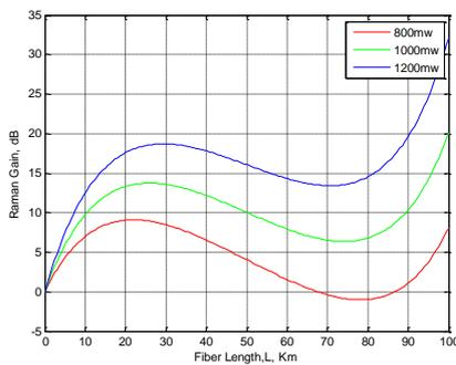
**Fig. 2** Raman gain against the fiber length with different pumping power for SMF
