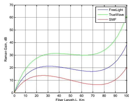
**Fig. 6** Raman gain against the fiber length with different fiber types at 1000mW pumping power
