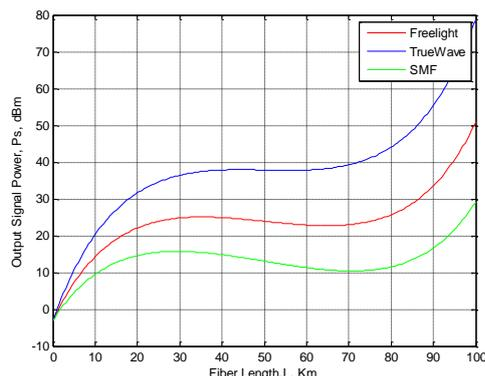
**Fig. 10** Output signal power against fiber length at 1200mW pumping power and -3dBm input signal power
