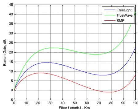
**Fig. 5** Raman gain against the fiber length with different fiber types at 800mW pumping power
