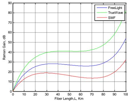
**Fig7.** Raman gain against the fiber length with different fiber types at 1200mW pumping power
