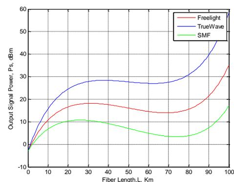
**Fig. 9** Output signal power against fiber length at 1000mW pumping power and  $-3\text{dBm}$  input signal power
