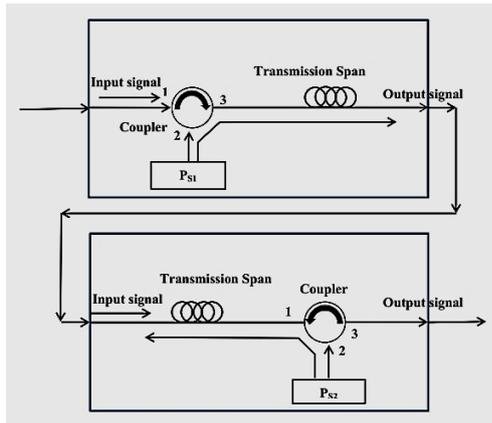
**Fig. 1.** Design model of Raman amplifier system scheme.
