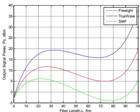
**Fig. 8** Output signal power against fiber length at 800mW pumping power and  $-3\text{dBm}$  input signal power
