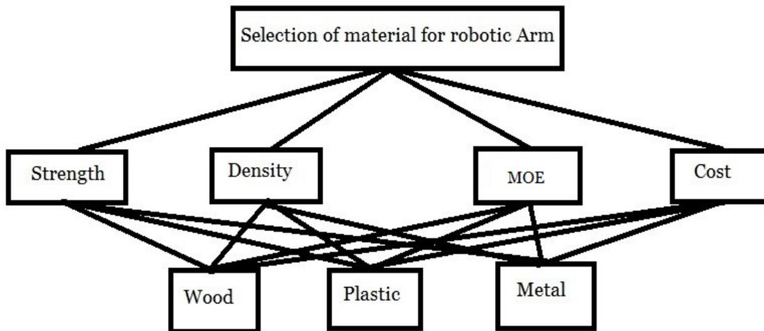
**Figure 2:** Decision Hierarchy for selecting material for frame of robotic Arm
