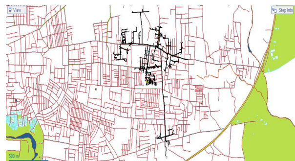
Fig. 4. Feeder Network Modelling Using CYMDIST 7.1
