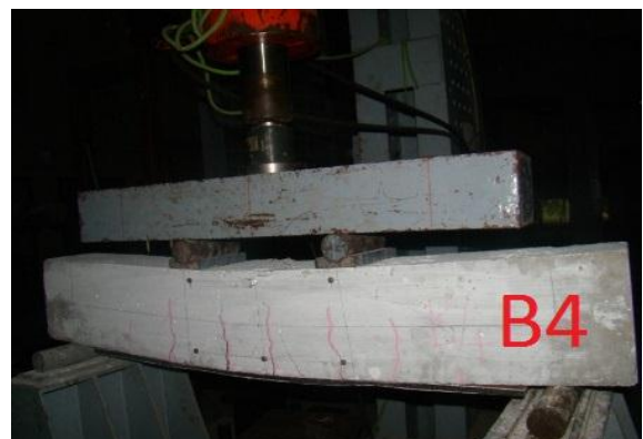
Figure 16. Failure of Beam B4
