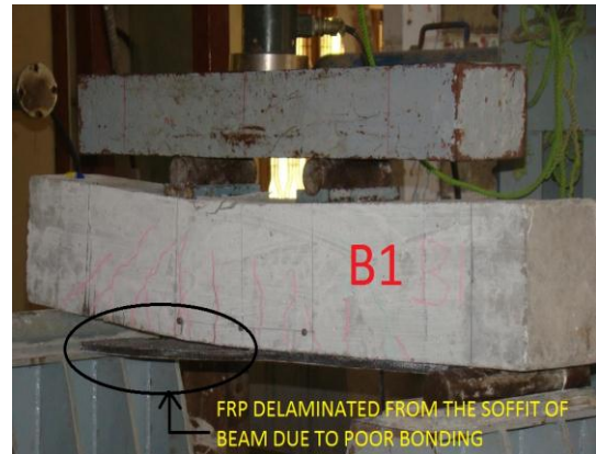
Figure 15. Failure of Beam B1
