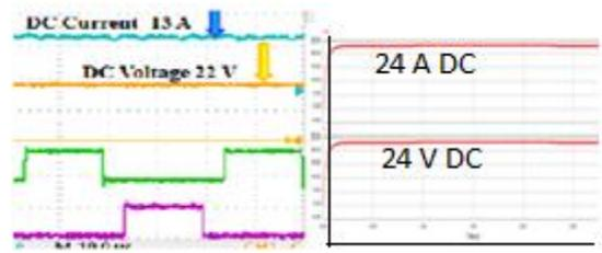
**Figure 32.** comparative results of DC voltage and DC current of converter with z-source across load at 50 kHz switching frequency (a) hardware result (b) simulation result
