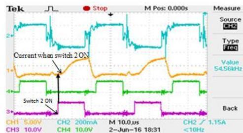
**Figure 21.** Transformer Secondary at terminal 2 when switch 2 is on for 45 % DR at 54.56 kHz switching frequency
