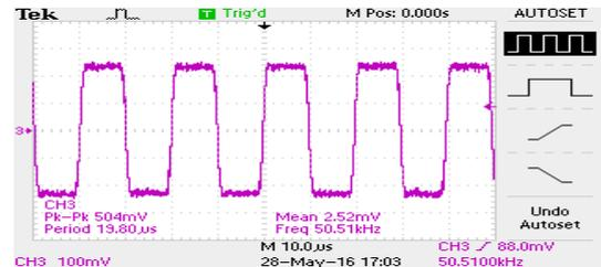
**Figure 17.** Transformer secondary voltage 5.04 V at 50.51 kHz switching frequency
