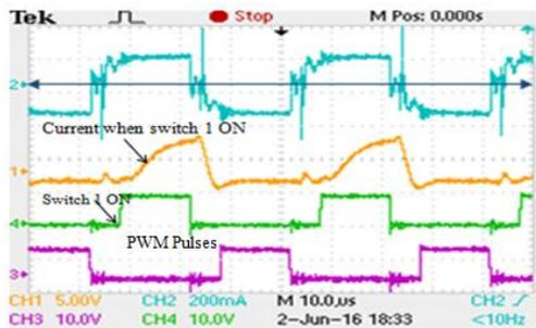
**Figure 20.** Transformer secondary current at terminal 1 when switch 1 is ON for 45% duty ratio, 50.25 kHz frequency.
