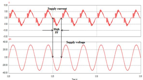
**Figure 7.** Source current and source voltage of z-source push-pull Converter resulting in near to unity power factor
