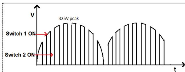
**Figure 3(a)** Expected output of input rectifier with z-source
