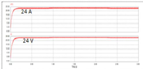
**Figure 9.** DC voltage and current waveform across the load
