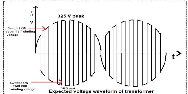
**Figure 3(b)** Expected Voltage envelop waveform of transformer with z-source without capacitor filter
