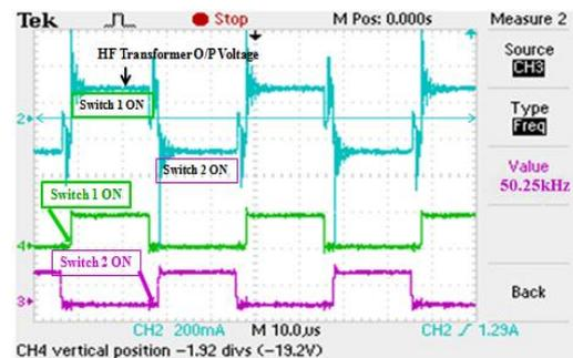
**Figure 19.** Output of Converter for 45% Duty Ratio with Load at 50.25 kHz
