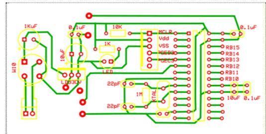
**Figure 11(a)** Printed Circuit Board for microcontroller dsPIC33EP256MC202
