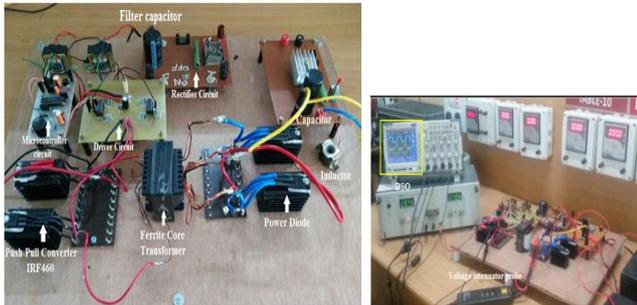
**Figure 14.** Complete Hardware and experimental set up of z-source push-pull high frequency high input power factor AC-DC converter
