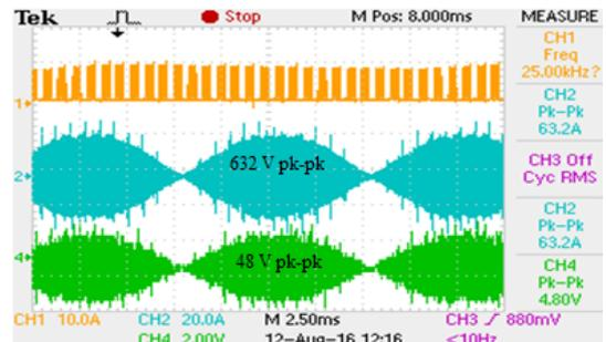
**Figure 24.** HF transformer input voltage 632 pk- pk and output voltage 48.0 volt with z-source
