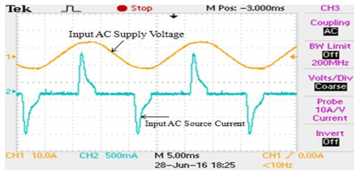
**Figure 29.** Source voltage and source current of conventional HF Push-Pull DC-DC converter at 50 kHz switching frequency w/o z-source
