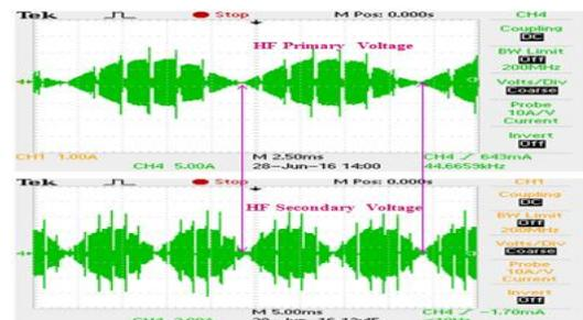
**Figure 25.** HF Transformer Primary and secondary voltage at 45 kHz switching frequency
