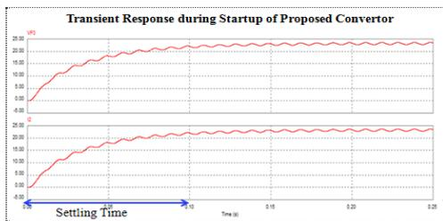
**Figure 10.** Transient Response during Startup of Proposed z-source AC-DC push-pull converter
