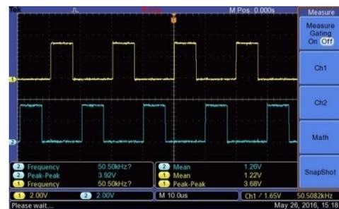
**Figure 12.** 50 kHz , 3.9 V pulses from control circuit.
