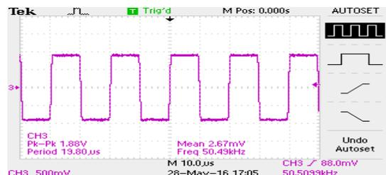
**Figure 18.** Transformer secondary voltage 18.8 V at 50.509 kHz switching frequency
