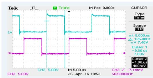
**Figure 15.** PWM Gate Pulses for 40.40 % duty ratio,  $\Delta t=8.0 \mu s$  At switching frequency of 50.508 kHz from driver circuit
