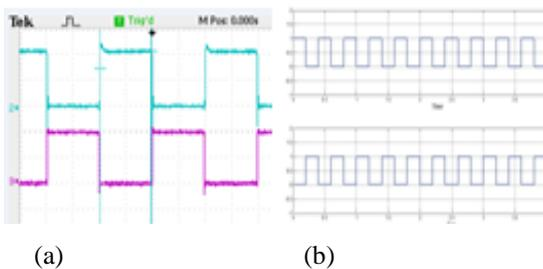
**Figure 30.** PWM Gate Pulses for 50% duty ratio for 50 kHz switching frequency (a)- Hardware waveform (b)- Simulation result
