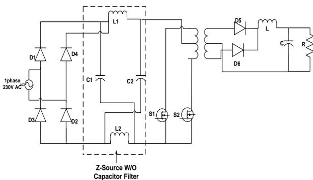
**Figure 2.** Circuit diagram ac/dc z-source push-pull converter
