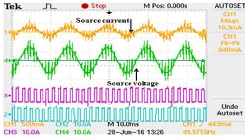
**Figure 27.** Source current and source voltage of the converter with z-source at 49.975 kHz switching frequency resulting in high input power factor
