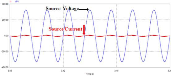
**Figure 8.** Source current and source voltage (230 V) with z-source push-pull Converter resulting in a high power factor near to unity.
