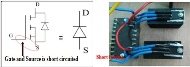
**Figure 13.** Connection Diagram of MOSFET (IRF460) as HF Power Diode
