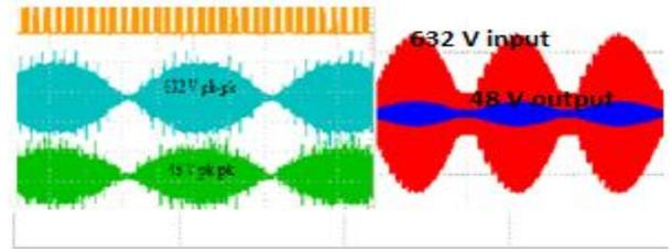
**Figure 31.** Comparative results of peak to peak input and output voltage envelop of converter with z-source (a) Hardware results (b) Simulation result
