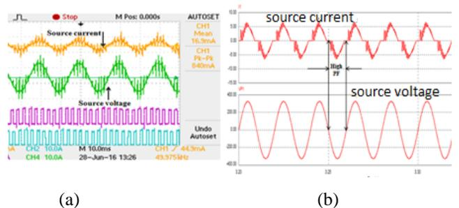
**Figure 33.** comparative results of Source current and source voltage of the converter with z-source at 49.975 kHz switching frequency resulting in high input power factor (a) hardware result (b) simulation result
