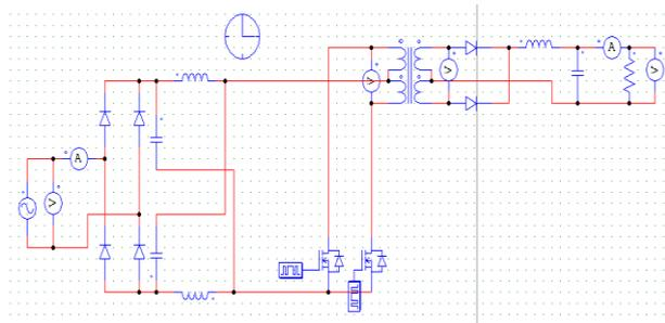
**Figure 4.** Simulation model of z-source Push-Pull converter
