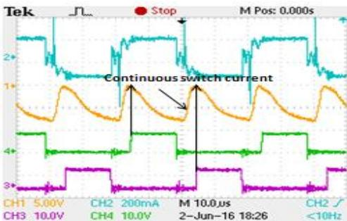
**Figure 22.** Continuous switch Current at terminal 3 (center tap terminal) of the transformer for 45% duty ratio at 50 kHz frequency
