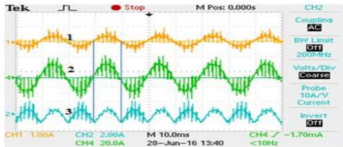
**Figure 28.** 1- Source current, 2- Source voltage 3- HF output rectifier current for switching frequency of 50 kHz. All are in phase
