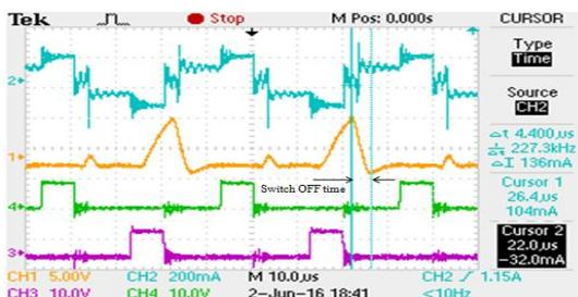
**Figure 23.** The turning off time of switch  $\Delta t=4.4 \mu$ s of push-pull switches
