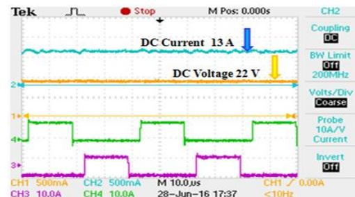
**Figure 26.** DC voltage and DC current of proposed converter with z-source across load at 50 kHz switching frequency
