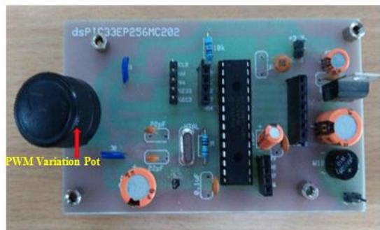
**Figure 11(b)** Hardware setup of microcontroller IC dsPIC33EP256MC202
