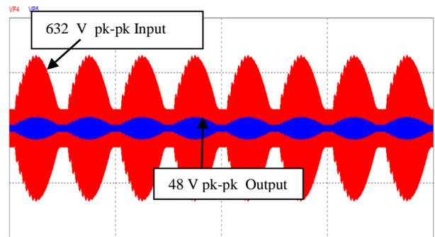
**Figure 5.** Input and output voltage waveform of HF transformer of z-source push-pull converter
