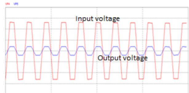
**Figure 6.** Zoom view of input and output voltage of High Frequency Transformer
