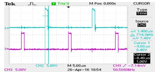
**Figure 16.** PWM Gate Pulses for 7.07 % duty ratio,  $\Delta t=1.4 \mu s$  At switching frequency of 50.508 kHz from driver circuit
