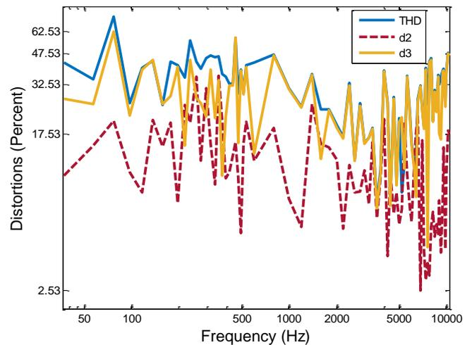
**Figure 4:** Experimental graphs of THD and harmonic distortion components  $d_2$  and  $d_3$
