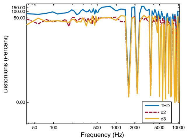
**Figure 5:** Estimated THD and harmonic distortion components  $d_2$  and  $d_3$  graphs ( $\lambda = 0.85$ ,  $MSE = 3.5381e+12$  and  $PVRP = 1.2478e+15$ )
