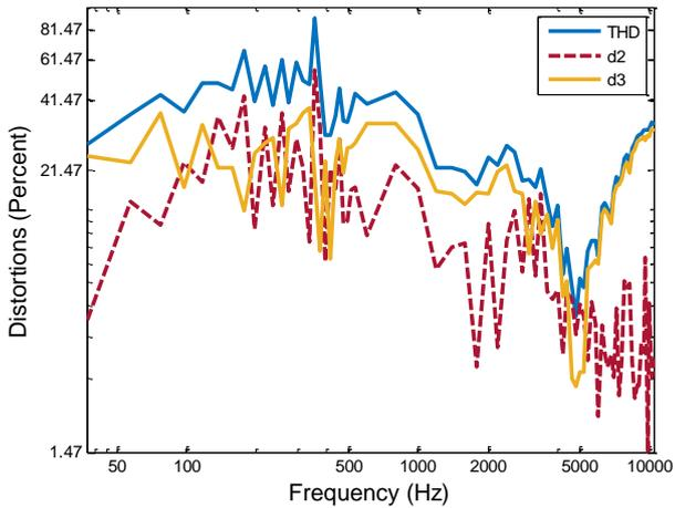
**Figure 6:** Estimated THD and harmonic distortion components  $d_2$  and  $d_3$  graphs ( $\lambda = 0.90256$ ,  $MSE = 0.0373$  and  $PVRP = 13.1876$ )
