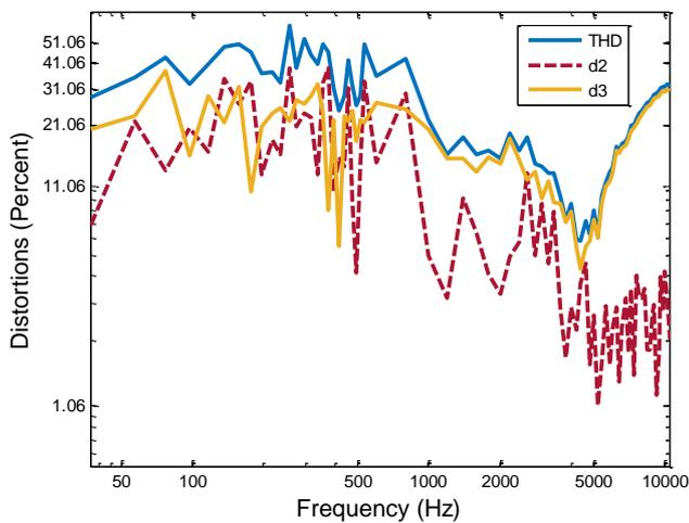
**Figure 8:** Estimated THD and harmonic distortion components  $d_2$  and  $d_3$  graphs ( $\lambda = 0.9414$ ,  $MSE = 0.0574$  and  $PVRP = 0.4626$ )
