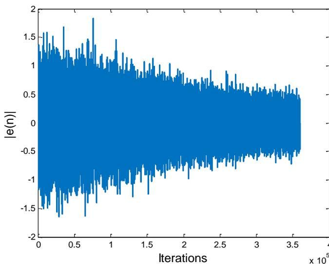
**Figure 2:** Error signal of the RLS AVF with  $\lambda = 0.99$
