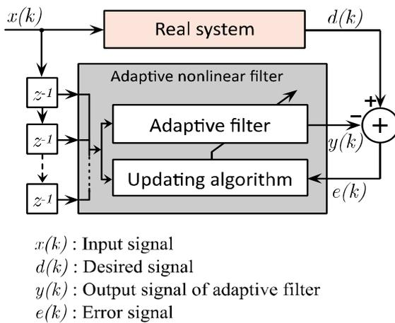
**Figure 1:** Diagram of system modeling using RLS AVF
