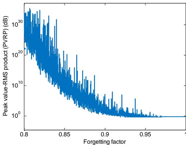
**Figure 3:** Peak Value-RMS Product (PVRP) vs. forgetting factor sweeping between 0.8 and 1, for third-order RLS adaptive Volterra filter with  $M = 2$ .
