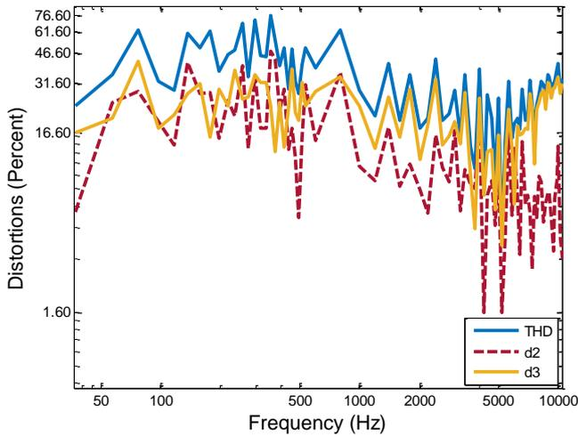
**Figure 7:** Estimated THD and harmonic distortion components  $d_2$  and  $d_3$  graphs ( $\lambda = 0.924975$ ,  $MSE = 0.0463$  and  $PVRP = 0.4146$ )
