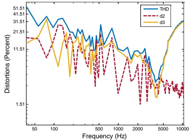
**Figure 9:** Estimated THD and harmonic distortion components  $d_2$  and  $d_3$  graphs ( $\lambda = 0.98$ ,  $MSE = 0.0961$  and  $PVRP = 0.6$ )
