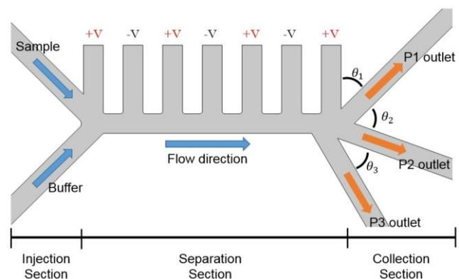
Figure 2. Schematic of the DE-FFF-based microfluidic device
