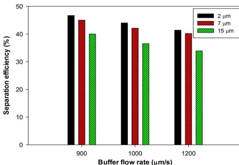
**Figure 5.** Separation efficiency of device with the effect of the buffer flow rates
