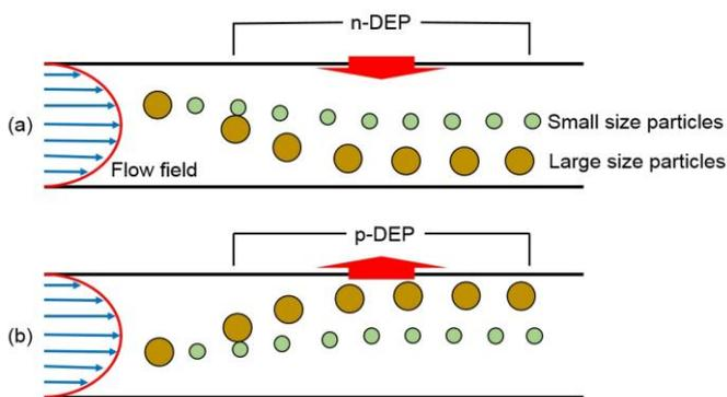
Figure 1. Field-flow fractionation with (a) n-DEP and (b) p-DEP techniques.
