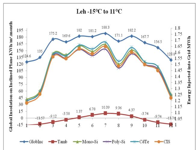
**Figure 1(a).** Monthly energy fed to the grid of the four simulated PV systems in Leh
