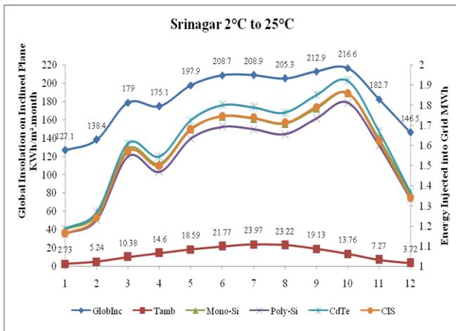
Figure 1(b). Monthly energy fed to the grid of the four simulated PV systems in Srinagar
