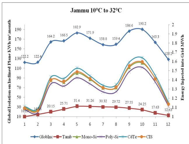
Figure 1(c). Monthly energy fed to the grid of the four simulated PV systems in Jammu
