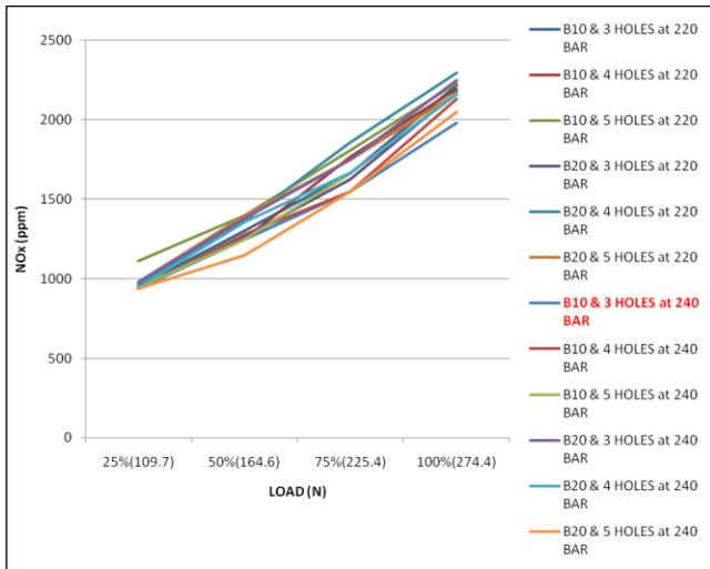
**Figure 7.** Variation of Load and Emission of Nitrogen Oxide ( $NO_x$ )
