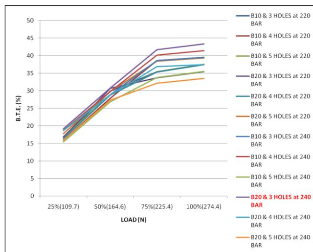
Figure 2. Variation of Load and Break Thermal Efficiency
