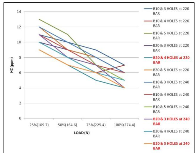
**Figure 6.** Variation of Load and Emission of Hydrocarbons (HC)
