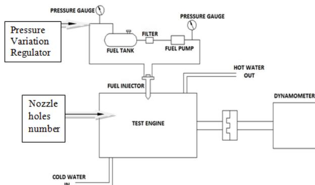
Figure 1. Experiment Set Up Line Diagram
