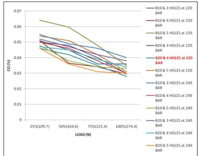
**Figure 5.** Variation of Load and Emission of Carbon Monoxide (CO)
