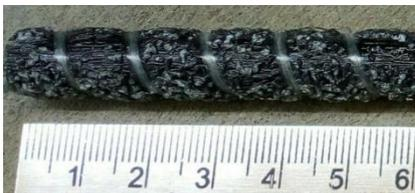
Figure 5. Short beam shear test specimen
