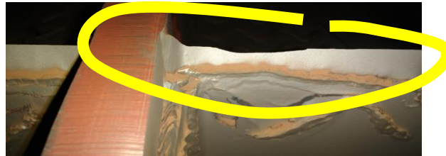
Figure 10. The impeller blades were wearing out at a faster rate
