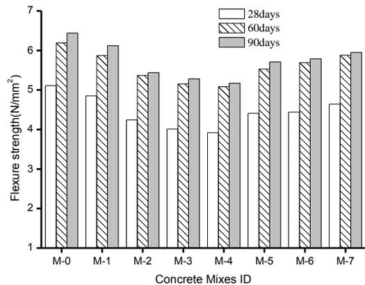
**Figure 8:** Flexure Strength of concrete mixes with various % of FA and GBFS
