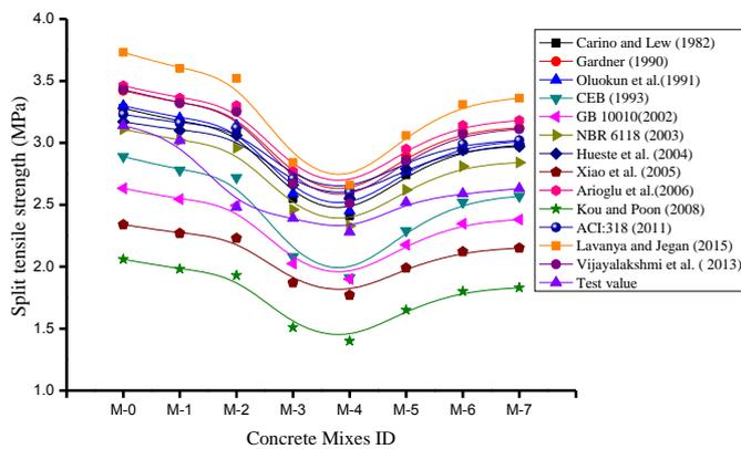
**Figure 7:** Line plot of split tensile strength obtained by various proposed models
