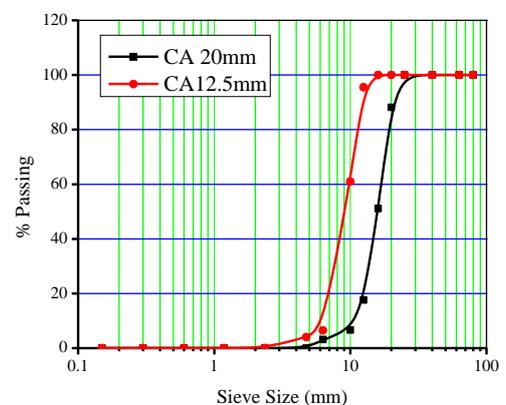
**Figure 2 :** Sieve analysis of coarse aggregates
