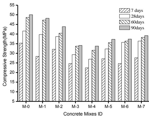
**Figure 5:** Compressive Strength of concrete mix with various % of FA and GBFS
