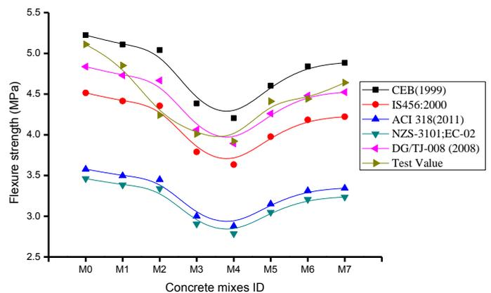
**Figure 9:** Line plot of flexure strength obtained by various proposed models
