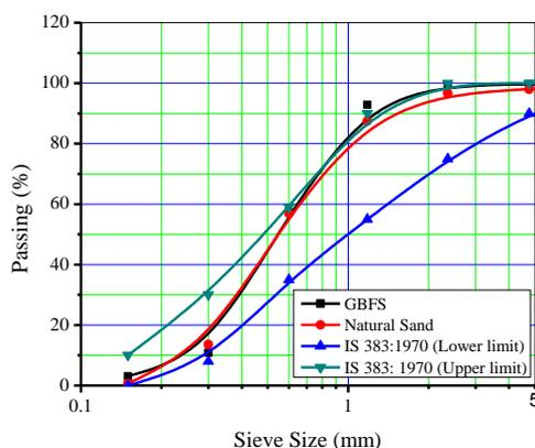
**Figure 1 :** Sieve analysis of fine aggregates (NS and GBFS)
