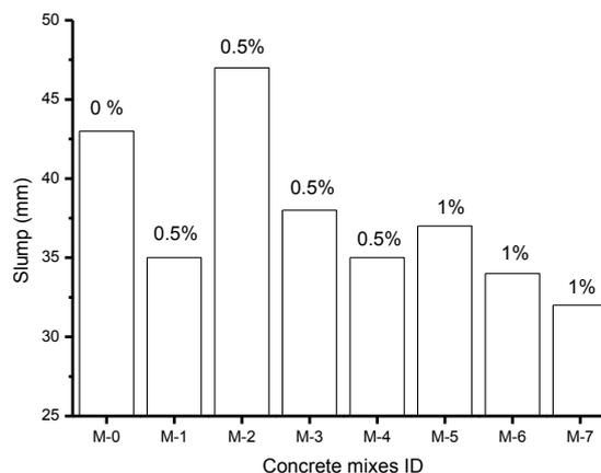
**Figure 4:** Slump and doses of super plasticizer versus concrete mixes
