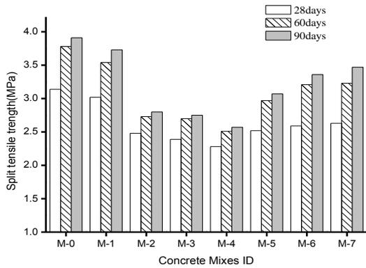
**Figure 6:** Split tensile Strength of concrete mixes with various % of FA and GBFS
