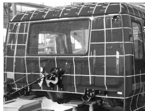
**Figure 5.** The measure dots of cab system's modal test
