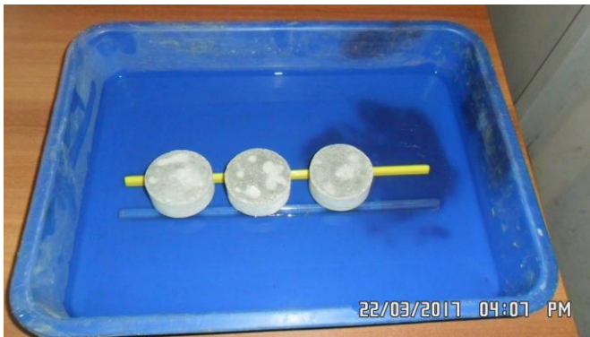
Figure 4. Sorptivity test set up
