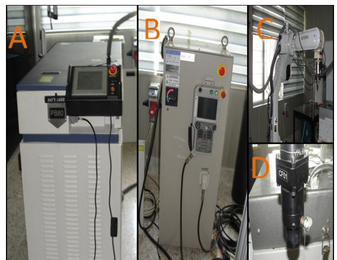
Figure 1. Nd-YAG Machine, 'A' the power supply, 'B' robot controller, 'C' & 'D' the robot arm
