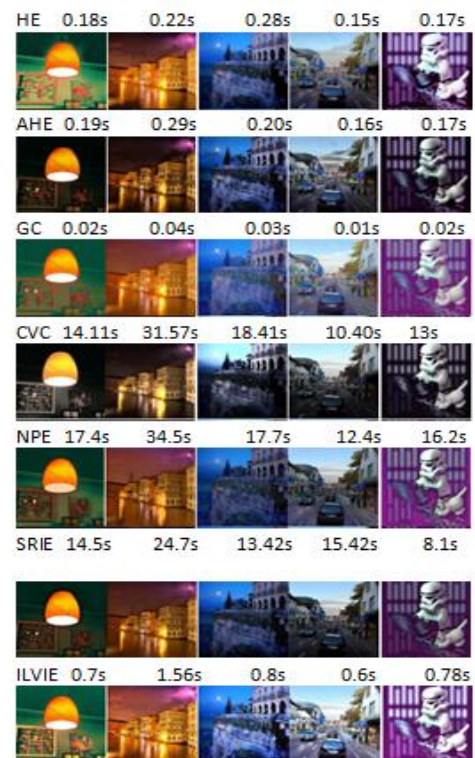
Figure 2. Computation time comparison and Quality of enhanced image between AHE, HE, CVC, GC and our technique
