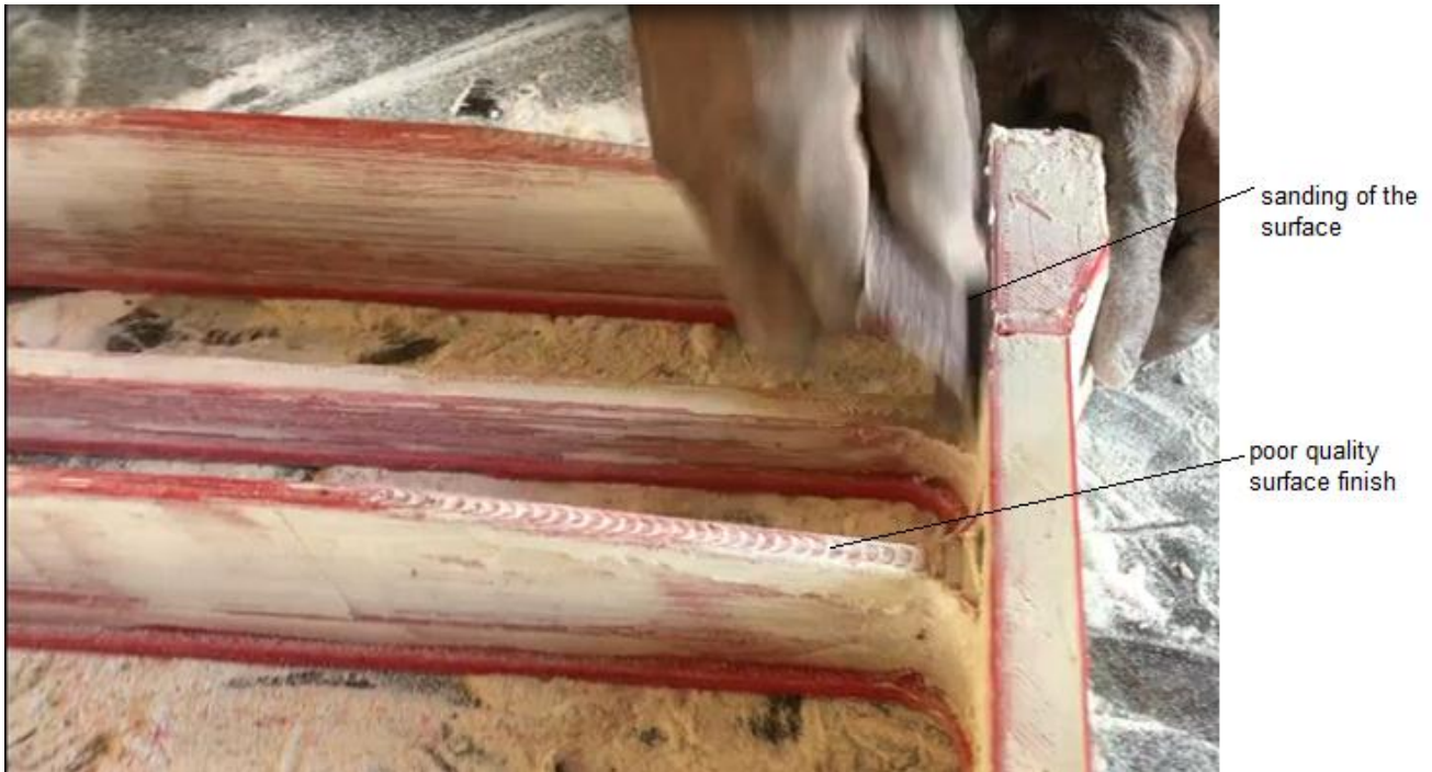
Figure 3. Poor surface finish of a FDM printed pattern that required post-treatment before moulding operation Source: [24]
