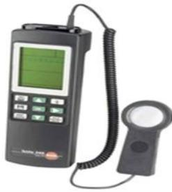
**Figure 5:** The portable light meter used for measurements [67].
