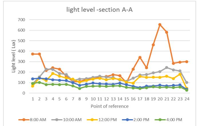
**Figure 7:** Measured light level at section A-A
