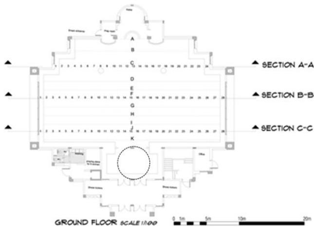
**Figure 6:** Plan of the tested mosques illustrating the points of readings.
