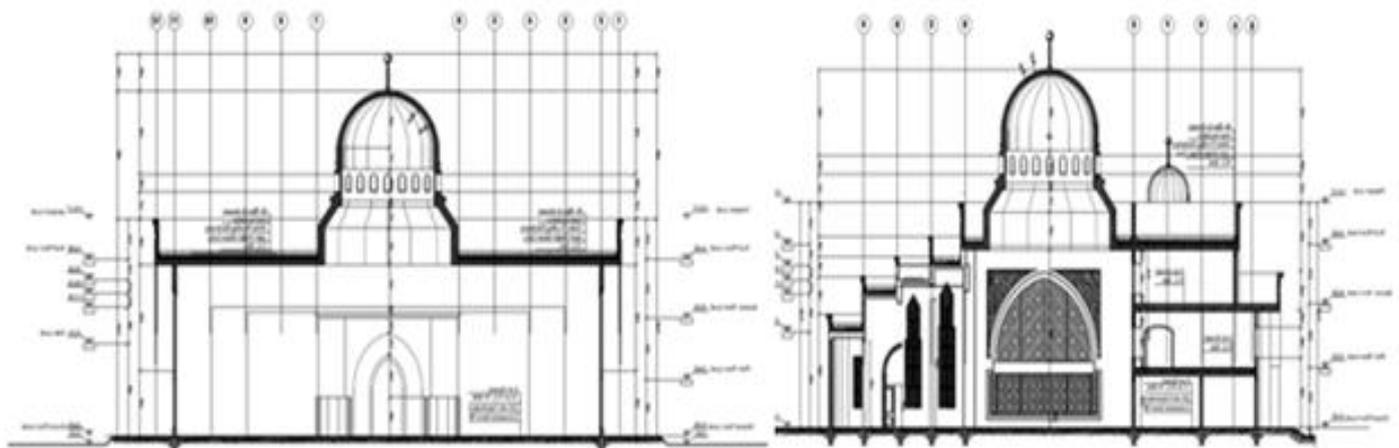
**Figure 4:** Sections through the mosques indicating the opening through the central dome.
