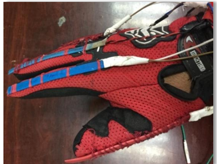
Figure. 3. Clever glove (flex sensor attach with glove)
