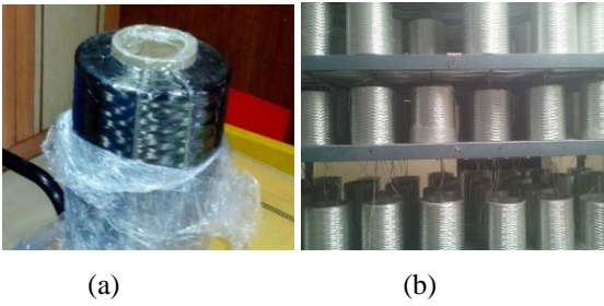
Figure 2. (a) Raw Carbon and (b) Glass fibres Rovings
