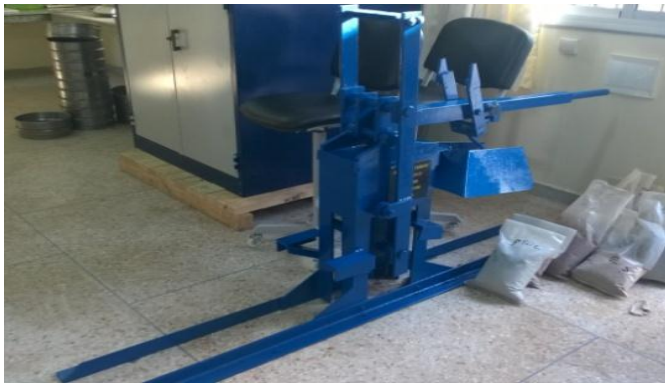
Figure 6: Press for CEB fabrication
