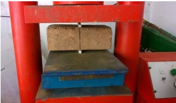
Figure 10 : Splitting tensile test
