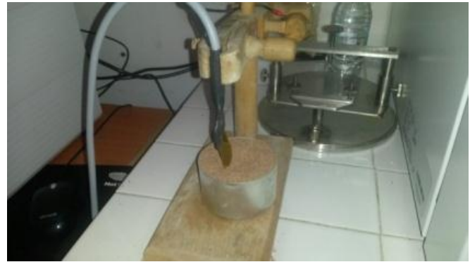
Figure 8: Measurement of thermal conductivity of PANS and soil
