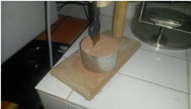
Figure 8: Measurement of thermal conductivity of PANS and soil
