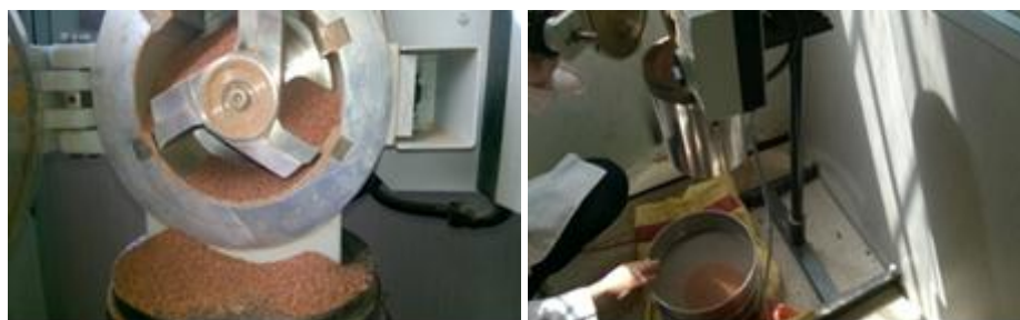
Figure 2: Crushing and sieving of PANS
