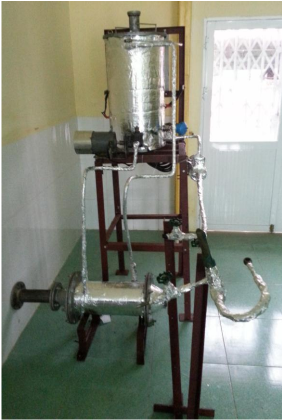
Figure 5. The SCO heating system by utilizing exhaust gas energy
