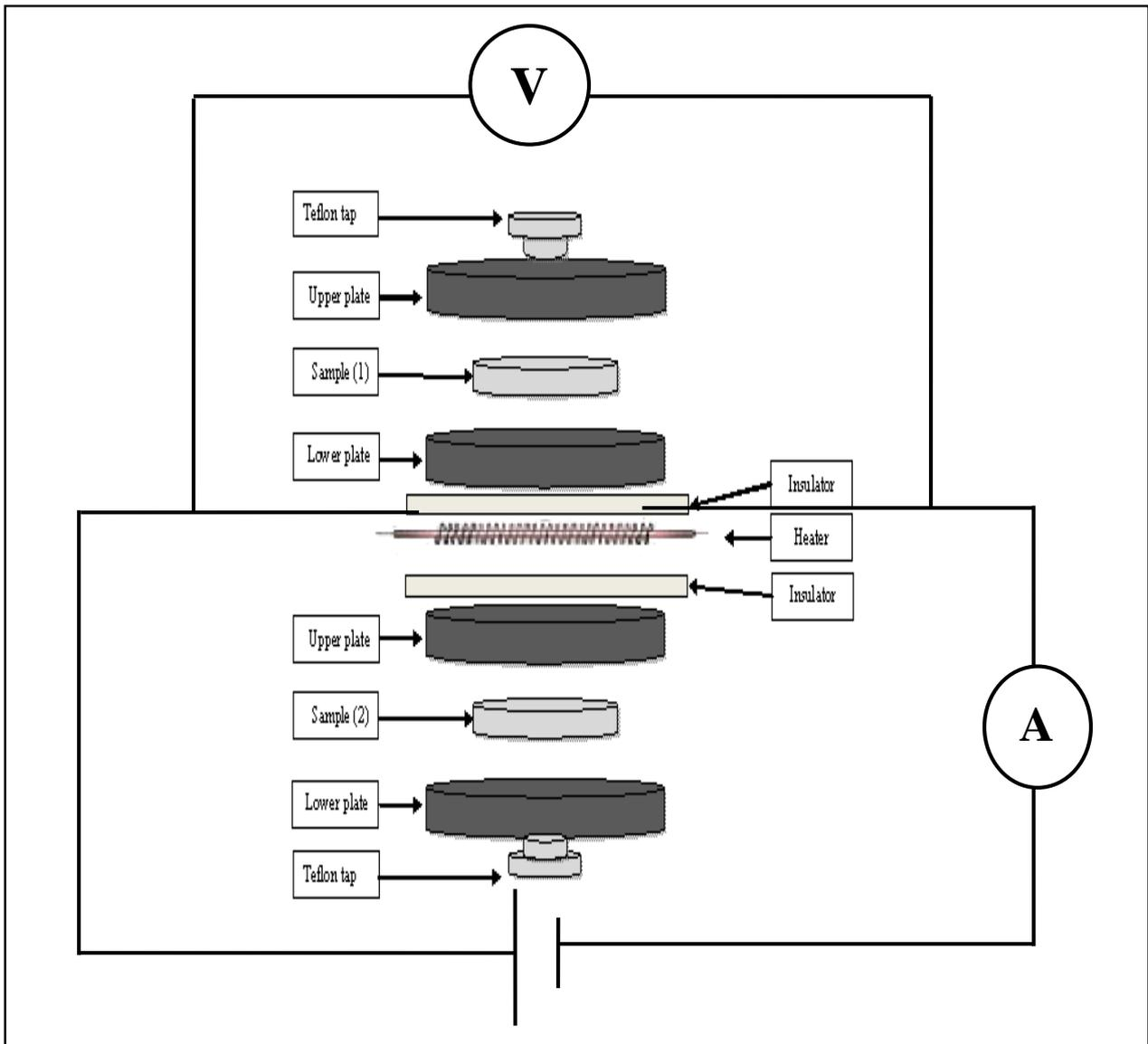
**Figure 2.3:** The circuit of thermal conductivity measurements
