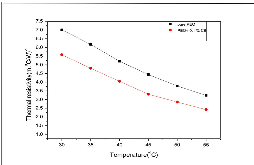
**Figure 3.3:** Variation of thermal resistivity ( $r = 1/k$ ) with temperature
