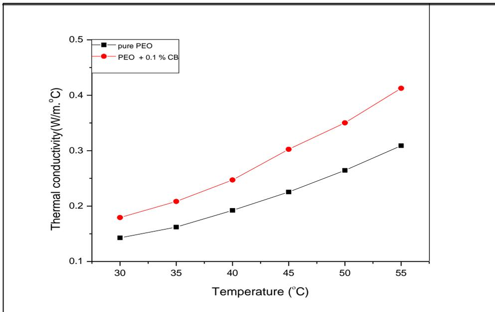
Figure 3.1: Thermal conductivity versus temperature for PEO/CB
