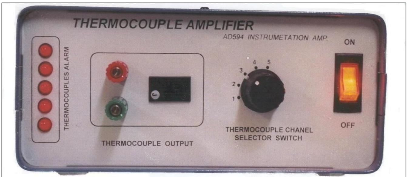
**Figure 2.1:** Thermocouple amplifier (AD594 instrumentation)
