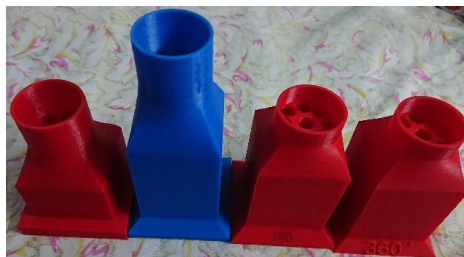
Figure 2: 3D Printed Ducts - 0°, 90°, 180°, 360°
