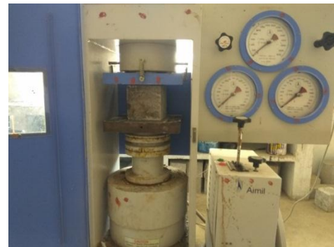
Figure 4.1 Compression testing machine
