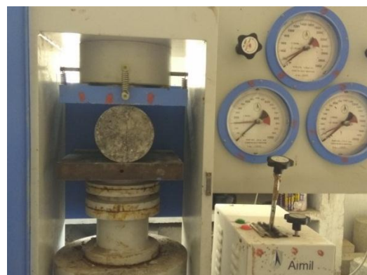
Figure 4.2 Split tensile testing machine
