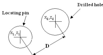
**Figure 3** Interference between vertical locator and drilled hole
