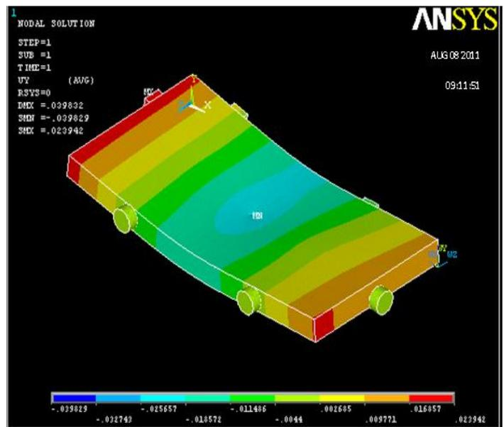
**Figure 6:** Deformed shape of the work piece
