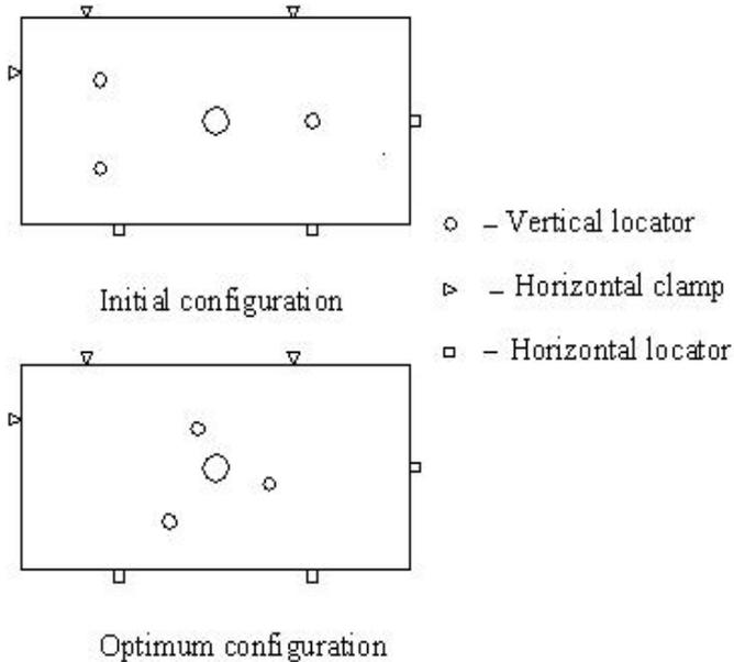
**Figure 7:** Schematic view of optimum configuration
