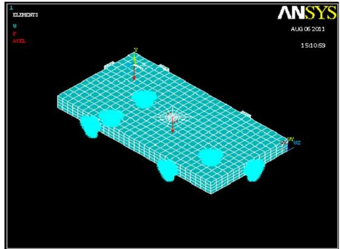
**Figure 5:** FEM model with applied boundary conditions
