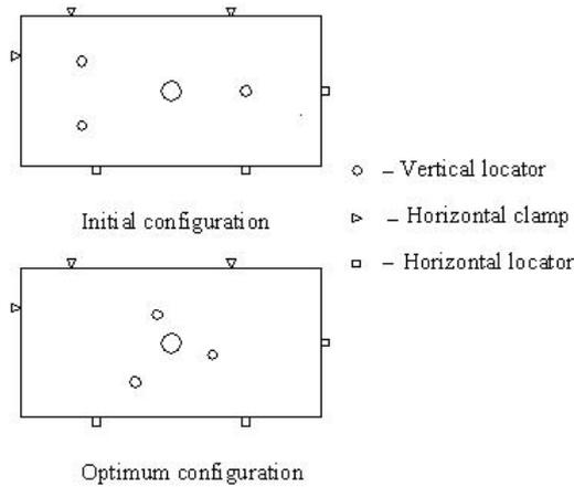
**Figure 8:** Initial and optimum fixture configuration for case
