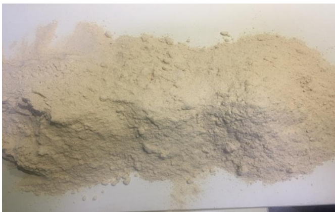
Figure 2. Shows the image of the remains of the quarries after drying and grinding
